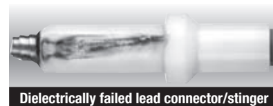
Dielectrically failed lead connector/stinger
