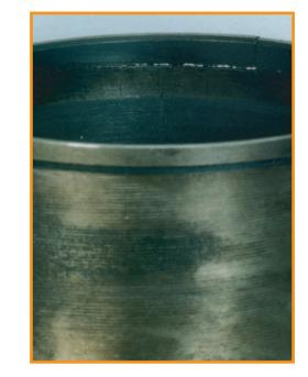
Symptom: Combustion gases ventilating to coolant, Engine noise, Eventual destruction of liner.
