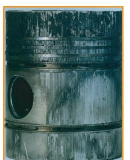
**Symptom:** Loss of power. Engine noise. Fumes from the engine breather.
