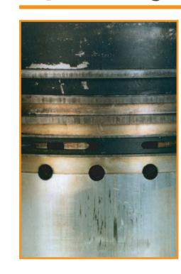
**Symptom:** Oil consumption, with possible fumes from engine breather. **Cause:** Excessive cylinder surface temperature. Marginal
