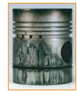
**Symptom:** Loss of power. Engine noise. Fumes from engine breather. **Cause:** Use of unsuitable liner sealing ring, use of
