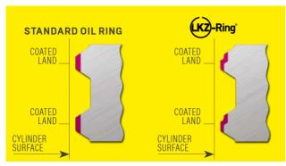
The asymmetric design of the LKZ-ring® ring reduces resistance when the piston is on the upward stroke reducing energy losses. When the piston is on the downward stroke the pressure more effectively returns the oil that lubricates the cylinder to the oil pan.
