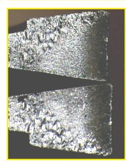
Cause: Ring overexpanded when fitting to piston. Discolouration at ring edge and polishing at fracture face indicate long time in service prior to failure. Remedy: Replace defective parts. Ensure piston and rings are fitted correctly. Use piston ring expanders during assembly to piston.
