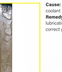
Cause: Overheating due to insufficient oil or coolant supply. Remedy: Replace defective parts. Check that lubrication and cooling levels are correct, and that the correct grade or lubricating oil has been used.
