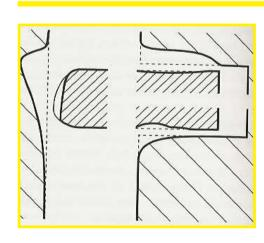
**Cause:** Shortage of lubrication. Incorrect choice o piston rings or cylinder liners. Cylinder distortion or inadequate cooling.
