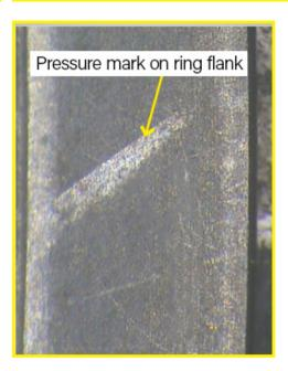
Cause: Dirt or debris in engine. Secondary damage due to overheating and seized piston(s). **Remedy:** Replace defective parts, clean engine, change oil, oil filter and air filter.
