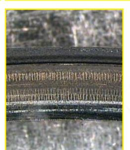
Cause: Dirt or debris in engine. Secondary damage due o overheating and seized piston(s). Remedy: Replace defective parts. Thoroughly clean engine and replace oil and filter.
