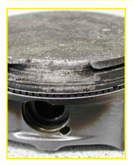
**Cause:** Overexpansion of ring when fitting the piston. Faulty fitting of piston or ring into engine block. Excessive pressure or worn piston grooves. **Remedy:** Replace defective parts. Ensure piston and rings are correctly fitted. Use piston ring expander to prevent overstressing of ring during assembly. Check if the piston grooves are to specification.
