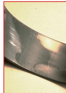
**Symptom:** Overplate wear only in the crown area of bearing shell towards the edge zones. Worn zones are shifted against each other in circumferential direction.
