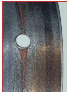
**Symptom:** Premature bearing wear. The internal surfaces may appear scratched and/or have embedded debris. Erosion may also be visible adjacent to an oil groove or hole.
