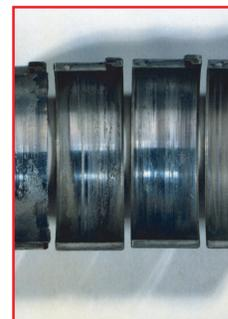
**Symptom:** Wiping or melting of the bearing surface which may progress to fatigue and destruction of the bearing material.
