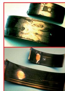
**Symptom:** Heavy local overplate wear. Local concentration of tin on steel back.
