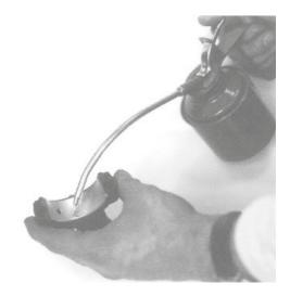
Fit bearings into the block and caps and allow oil to run over the bearing. Do not use a finger to wipe oil around the bearing.
