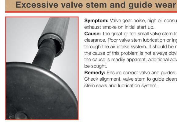
Symptom: Valve gear noise, high oil consumption, exhaust smoke on initial start up. Cause: Too great or too small valve stem to guide clearance. Poor valve stem lubrication or ingress of dirt
