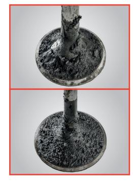
**Symptom:** Poor starting. Loss of power. Blue smoke from exhaust (when throttle closed). Cause: Excessive clearance between valve stem and guide. Valve stem seal failure or wear. Excessive oil supply due to blocked drainage paths. Incorrect grade of lubricating oil used.
