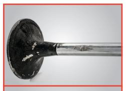
Symptom: Poor performance due to low compression. Mechanical breakage due to sticking valves. Cause: Marginal lubrication from inadequate valve to stem clearance, causing scuffing or metal transfer. This may ream out the valve guide leading to the second cause, excessive oil from too great a clearance carbonising on the stem to cause sticking.
