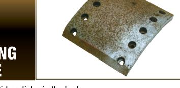
• Dirt particles in the brake
