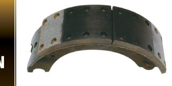
• Drum diameter is larger than lining radius Bedding-in period for the lining was too short
