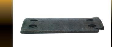
Wrongly adjusted or worn axle bearings
