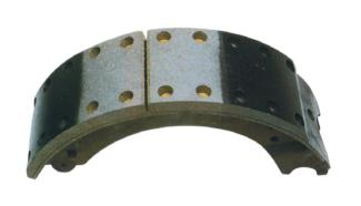
• Lining radius is larger than actual drum diameter Bedding-in period for the lining was too short
