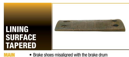
Distorted brake shoe or brake drum turned on taper **EFFECTS**
