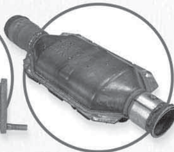
OVERHEATED SUBSTRATE / DISCOLORED SHELL
